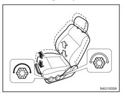
To adjust the height of the driver's seat cushion, turn the knobs located on the outboard side of the seat cushion.
